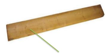
Asbestos fibres can adhere to timber planks and unsealed plywood and platforms
